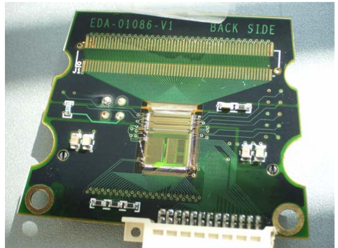
Figure 2: VFAT mounted on a gas sensor hybrid. The chip and bond wires are protected from damage by a protective cap (not shown).
